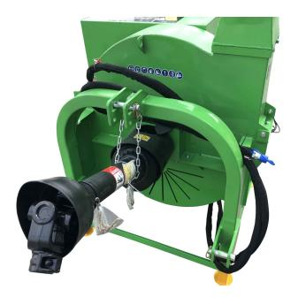
PTO shaft with adjustable friction clutch **Included**
